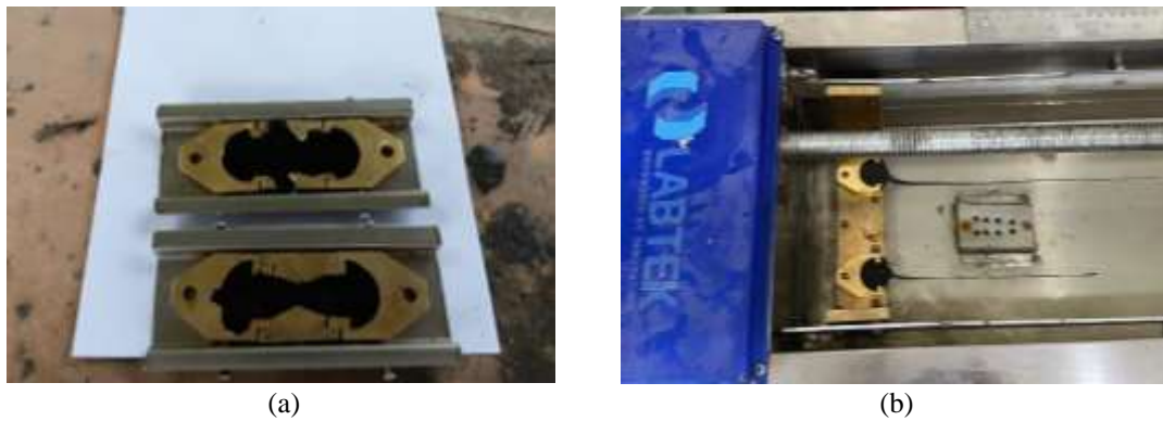
Gambar 9: (a) Sampel Bitumen/Aspal (b) Mesin Daktalitas
