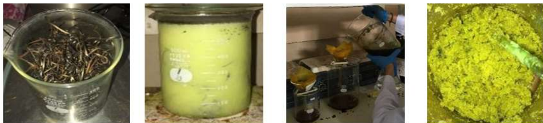
Fig. 1: The process of producing \text{FeCl}_3 coagulant from scrap iron from a lathe workshop
