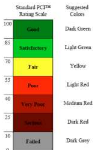
Gambar 2. Rating Kondisi Perkerasan Berdasarkan Nilai Pavement Condition Index (PCI)
