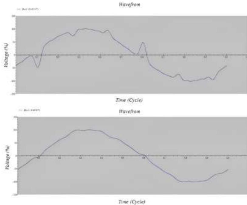
**Fig. 8:** Differences in Voltage Waveform Shape Before Filter Installation above
