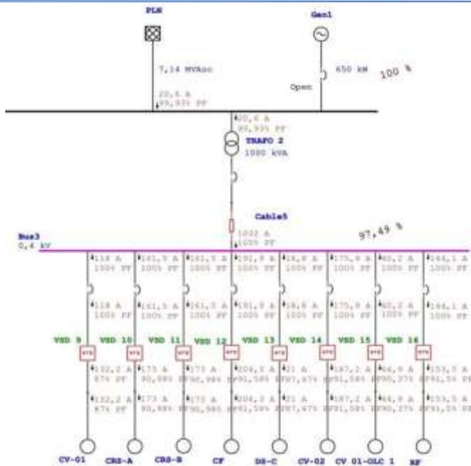
Fig. 6: The results of the load flow simulation for PT. BSSR
