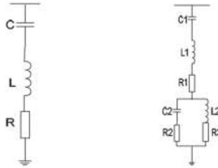
**Fig. 4:** Topology of tuned filter a. Single Tuned Filters dan b. Double Tuned Filters
