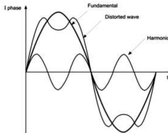
**Fig. 1** : The distorted waveform
