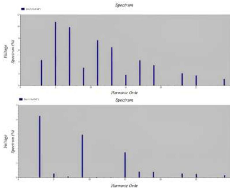
**Fig. 9:** Spectrum of Voltage without Filter above and with Filter below
