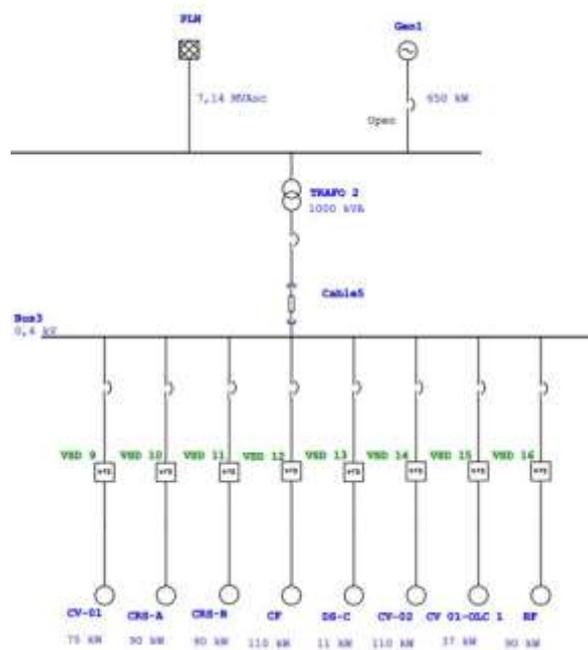
**Fig. 5:** Design of the electrical one-line diagram
