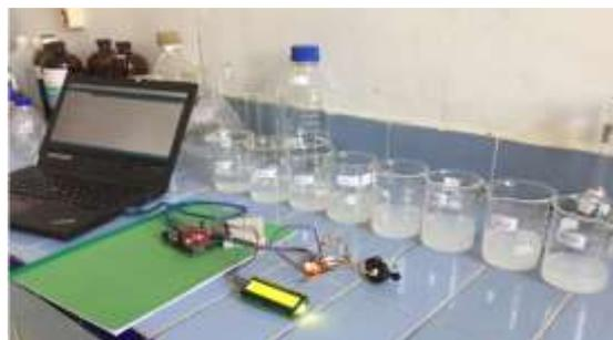
**Gambar 3.** Proses kalibrasi sensor turbidity
