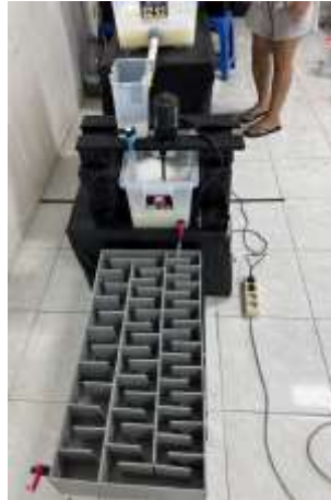
Gambar 2. Proses Koagulasi Mekanik - Flokulasi baffle channel
