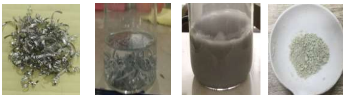
Figure 1. Zinc waste, zinc waste washing with hydrochloric acid, synthesis of zinc sulfate, and zinc sulfate crystals
