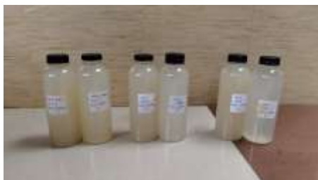
Figure 6. Comparison of Wastewater Before and After Treatment with Andosol Soil Type
