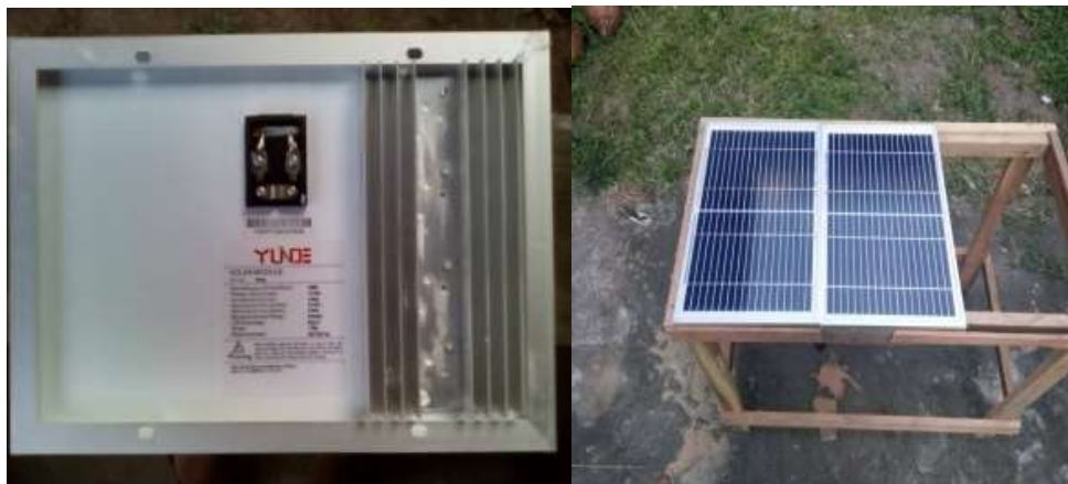
Fig. 3: Installation of solar modules on brackets and placement of heatsinks on solar modules
