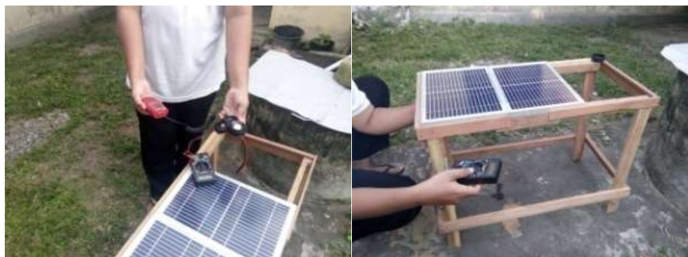
Fig. 4: Measurement of temperature, irradiation and output voltage
