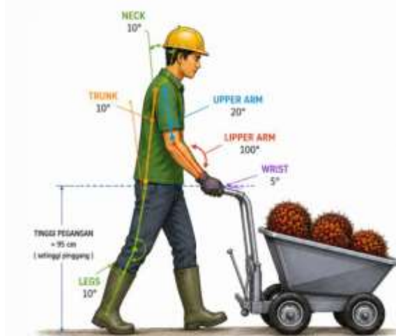
Figure 2. Working Posture After Using the Proposed Hydraulic Trolley
