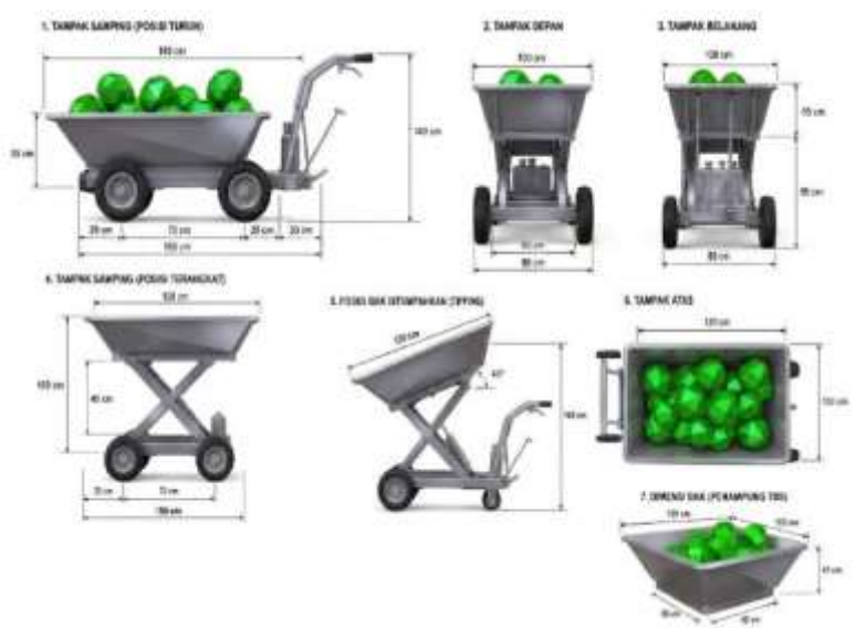
Figure 1. Proposed Hydraulic FFB Transport and Dumping Trolley
