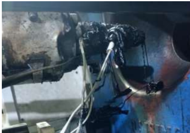
Gambar 3. Heater Nozzle terkena lelehan material
