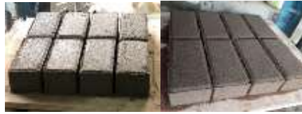
Gambar 1. Paving Block 0% Cocopeat dan Paving Block 10% Cocopeat Sumber: Riset, 2023
