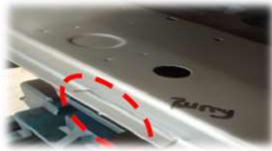
Gambar 1. Defect Burry pada Member Floor Side Inner LH
