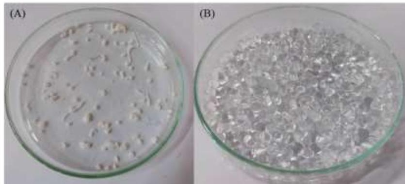
**Figure 2.**  $\kappa$ -carrageenan beads (A) dry (B) after contact with water for 24 hours
