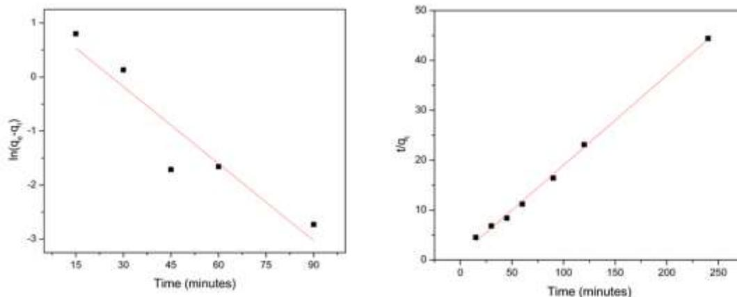
**Figure 4.** Linear fitting for adsorption kinetics (a) pseudo-first order kinetics (b) pseudo-second order kinetics of adsorption of Pb(II) on refined  $\kappa$ -carrageenan beads
