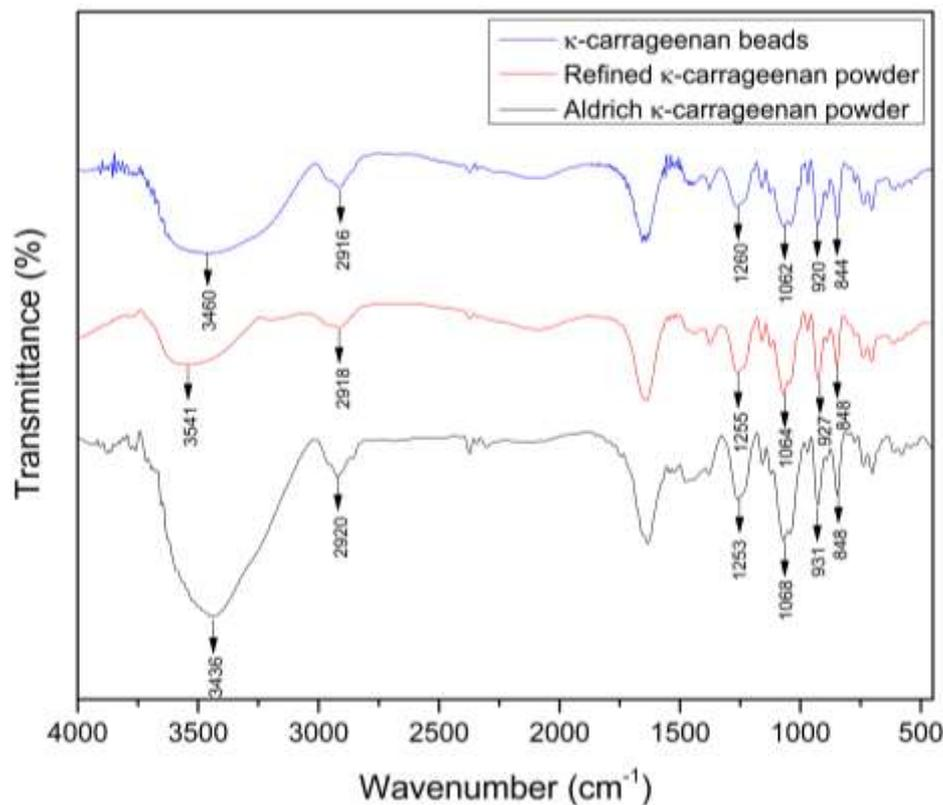
**Figure 1.** FTIR spectra of  $\kappa$ -carrageenan powder and  $\kappa$ -carrageenan beads.
