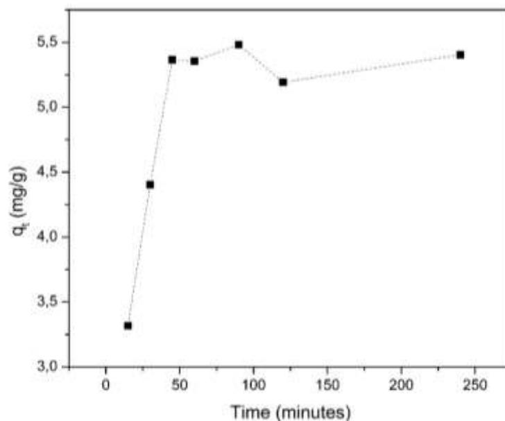
**Figure 3.** Effects of contact time on adsorption of Pb(II) on refined  $\kappa$ -carrageenan beads
