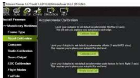
Figure 14. Pixhawk Accelerometer Testing
