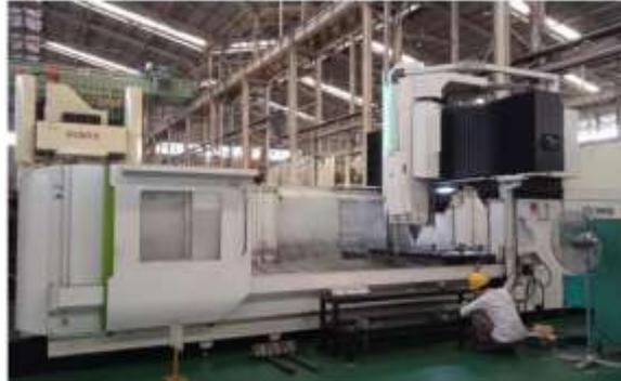
**Gambar 8.** Proses *Machining Lower Die*
