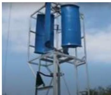
**Gambar 4.** Turbin Savonius
