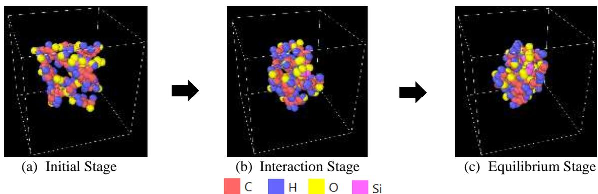
**Fig. 4:** Visualization of Interaction between Unsaturated Polyester and Glass Fiber in Molecular Dynamics (MD) Simulation
