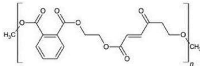
**Fig. 2:** Unsaturated Polyester Molecule Structure [9]
