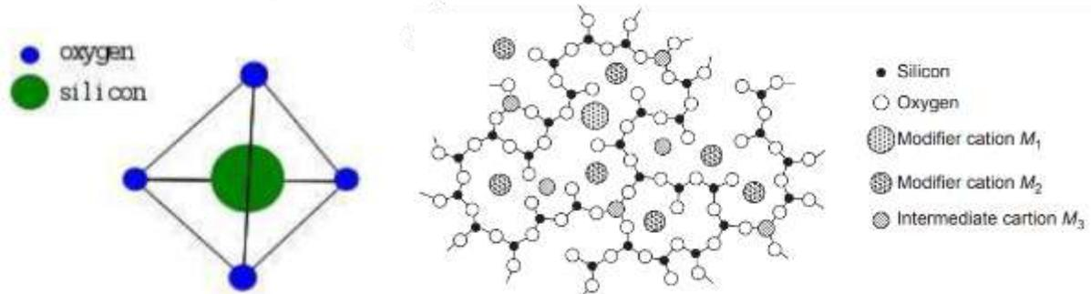
Fig. 3: Three-Dimensional and Two-Dimensional Glass Fiber Molecule Structure [17], [18]
