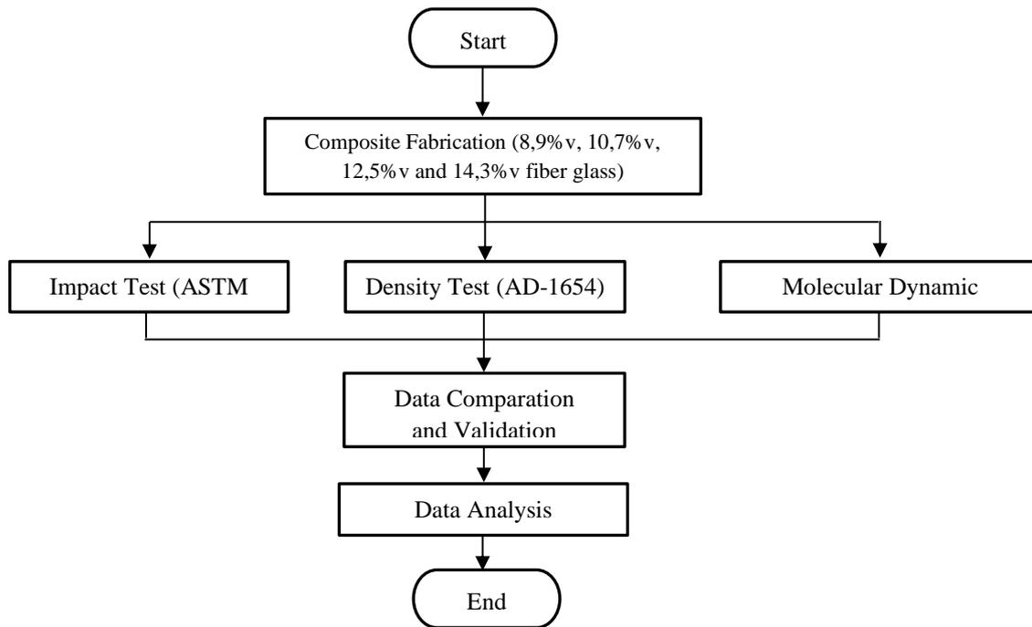
**Fig. 1:** Flowchart of Experimental and Simulation Methodology for Unsaturated Polyester/Glass Fiber Composites
