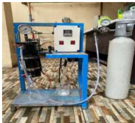
Gambar 2. Rangkaian Alat Metanasi CO 2 tipe Fixed Bed Reactor (2024)
