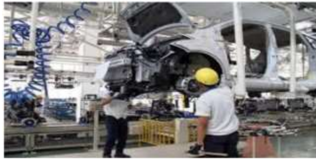
Figure 2. Installation of the front suspension on the car/unit
