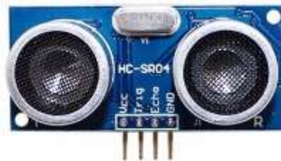
Fig. 2: Ultrasonic sensor HC-SR04 module [9]
